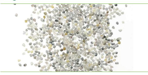
Blocky angular Boart provides the base for this gauge material. This material is mechanically treated in-house to remove brittle stones and thus increase the overall strength. This product was designed for use as a gauge keeper in a variety of bit types and sizes. In maintaining the gauge size the inherent characteristics of shape and toughness are utilized to greatest advantage.
